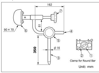
Note: Clamp for round bar is shown in the figure above.
